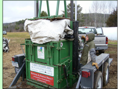
Compressing the Plastic into Bales. [Essex County]
